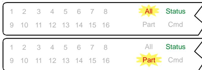
2. Enter your passcode to turn the system off. Once the system is off, the Command Center turns the All On indicator or the Part On indicator off.
